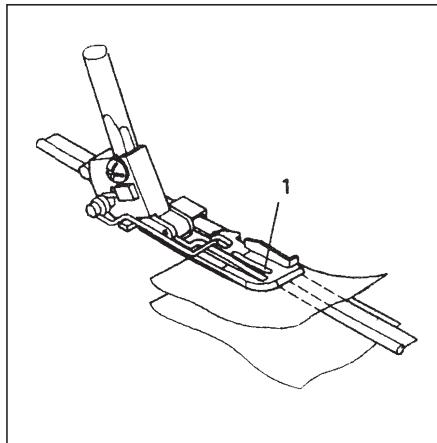
The Cording Foot is used for sewing piping (cording) between two layers of fabric in one easy operation.
